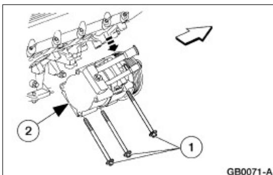
5. Remove the (CKP) sensor bolt and the crankshaft position sensor (CKP sensor) (6C315)
